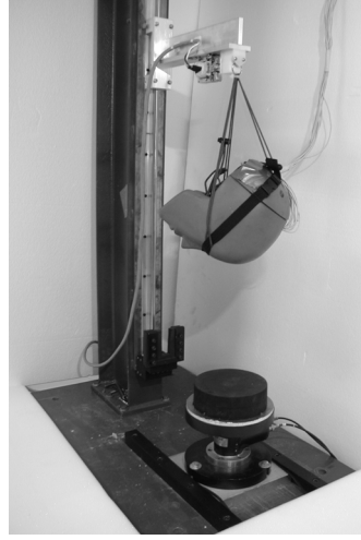
Fig. 1 – Hybrid III headform on drop assembly with target
